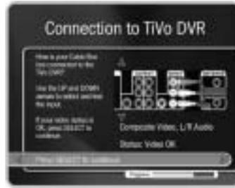
\* Use the UP/DOWN arrows until the picture of the DVR matches the cable connection you used to connect your satellite or cable box. When the video status below the picture says “Video OK,” press SELECT to continue. If the video status says “No Video,” double-check that the video cable is firmly connected to the DVR and that you have selected the correct type of video cable.
